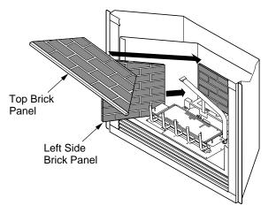
Figure 39 - Installing Left Side and Top Brick Panels
